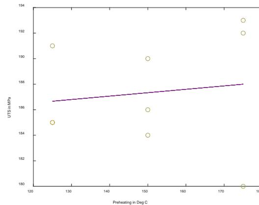
**Fig 6: Relation between UTS and preheating temperature**
