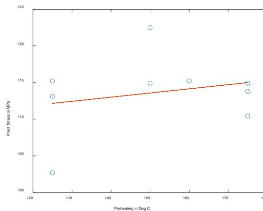
**Fig 7: Relation between Proof stress and preheating temperature**
