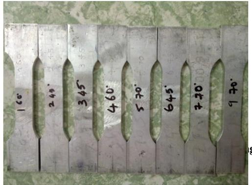
Fig 2: Tensile test samples
