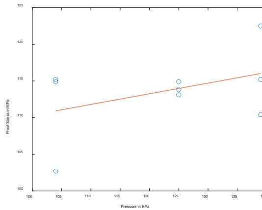
**Fig 4: Variation of Proof Stress with the variation of gas pressure**
