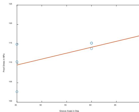
**Fig 6: Relation between Proof Stress and groove angle**
