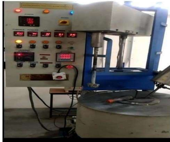
Fig3: Stir Casting Machine
