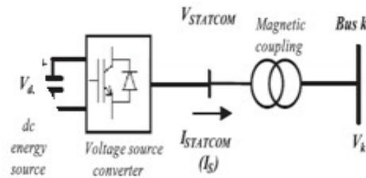
Fig.1 Single line STATCOM Power Circuit
