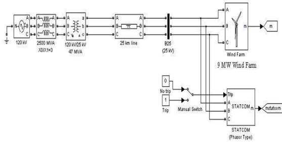
Fig.3. Simulink diagram of grid connected wind farm
