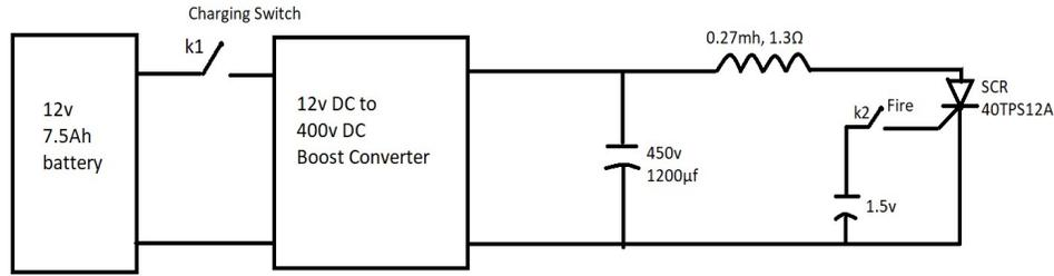
Fig 3: Firing Circuit
