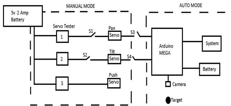
Fig 2: Servo control system
