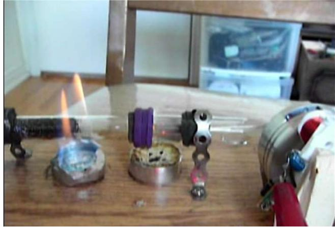
**Fig 1. Thermo acoustic engine using heat source**
