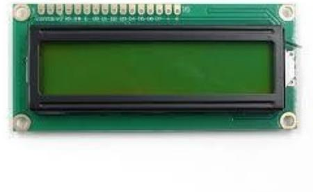
**Fig-3: 16X2 LCD Display**
