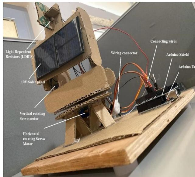
**Figure.4: Proto Type model of Dual Axis Solar Tracker**
