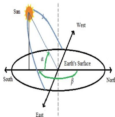
**Figure.1: Demonstration of Solar angles [i] Altitude angle ( $\alpha$ ), [ii] Solar Azimuth angle ( $\beta$ ).**
