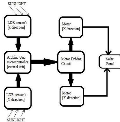
**Figure.2: Dual Axis Solar Tracker Hardware Diagram Block Implementation.**
