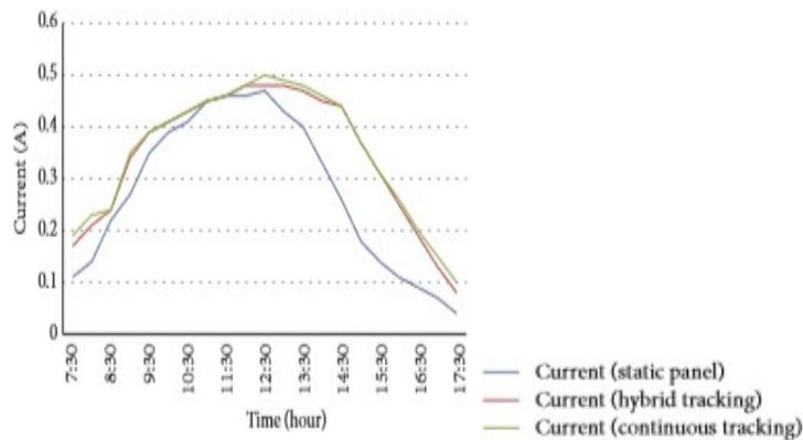
**Figure.5: Demonstration of Time v/s Current curve for Dual axis tracking system, Single-axis tracking system, and Static solar panel.**
