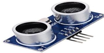
Fig. 5 Ultrasonic sensor
