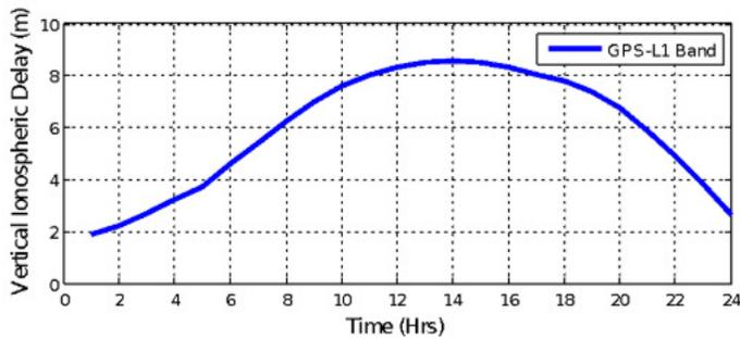
Figure 1 Vertical Ionospheric Delay in L1 band
