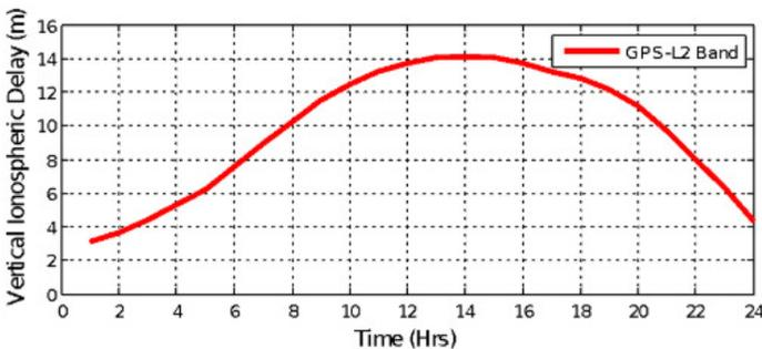
Figure 2 Vertical ionospheric delay in L2 band
