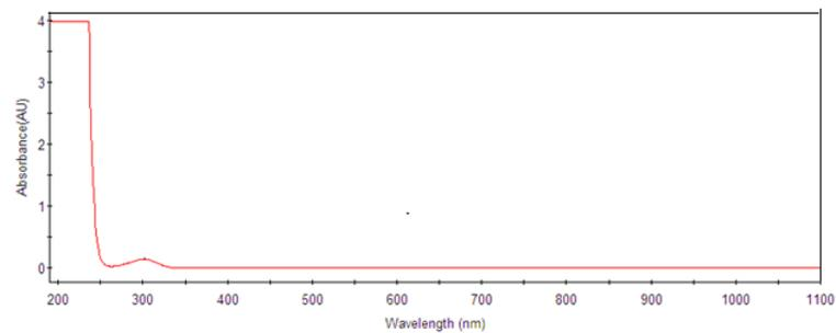
Fig. 5. UV-visible absorbance spectrum of LHSC crystal
