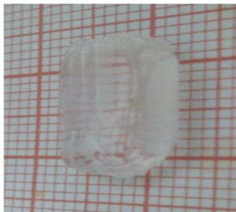
Fig.1: The grown crystal of LHSC
