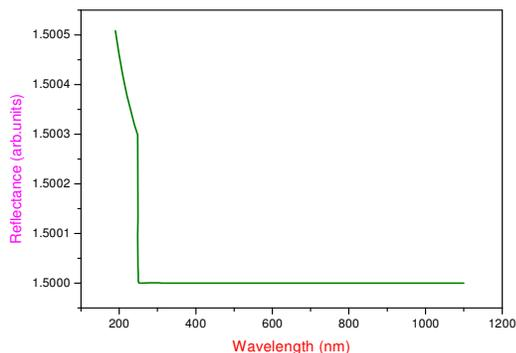
Fig. 7. Variation of reflectance with wavelength for LHSC crystal
