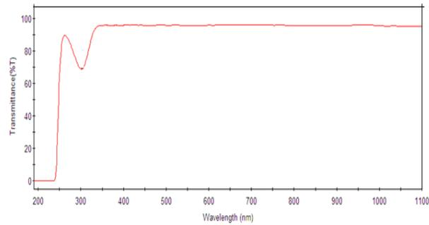
Fig. 4. UV-visible transmittance spectrum of LHSC crystal
