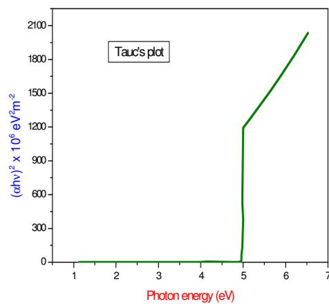
Fig. 6. Tauc's plot for LHSC crystal
