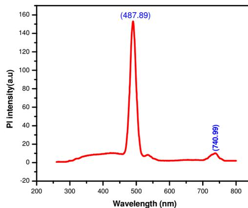
Fig.10: Photoluminescence spectrum of LHSC crystal
