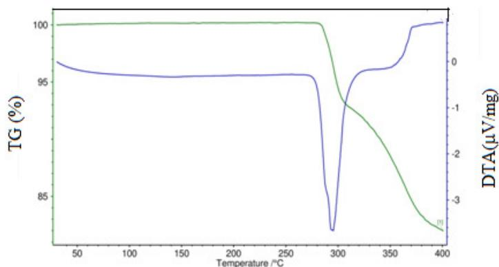
Fig.8: TG/DTA thermal curves for the grown LHSC crystal
