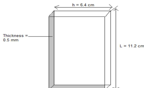
Figure1: Layout of rectangular copper fin of proposed heat exchanger.
