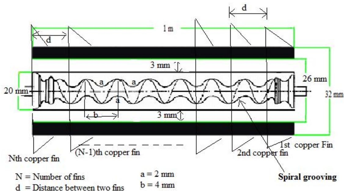
**Figure 3:Layout of internal spiral groove concentric tube with rectangular copper fin heat exchanger with different distance.**
