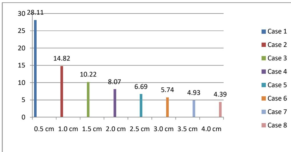
Figure 5. Graph between overall fin effectiveness (y-Axis) and distance between fins (x-Axis).
