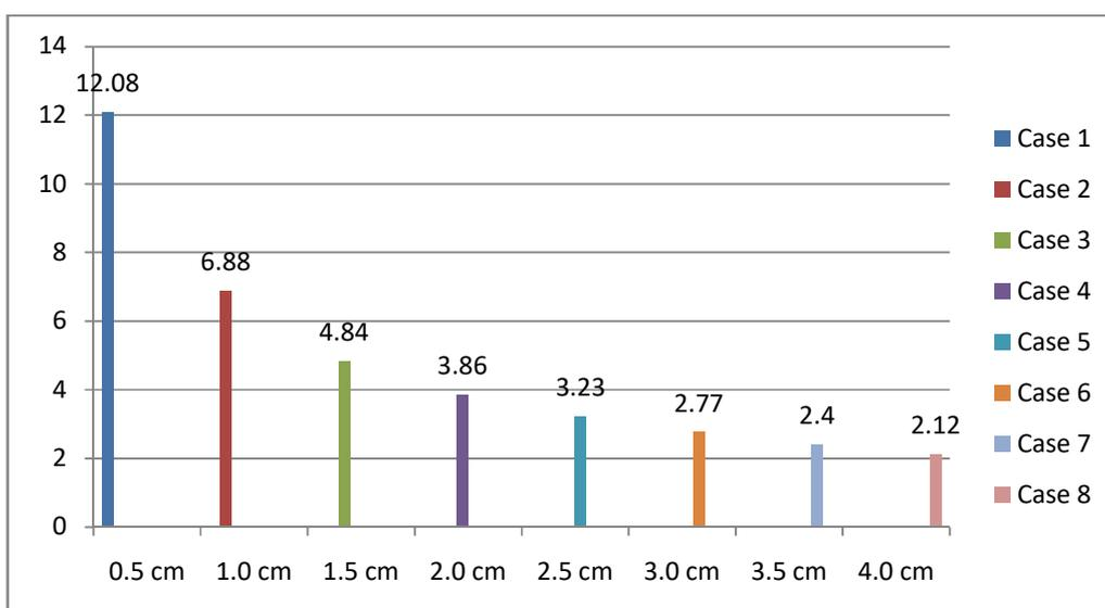
Figure 6. Graph between effectiveness of cross flow ACHE (y-Axis) and distance between fins (x-Axis).
