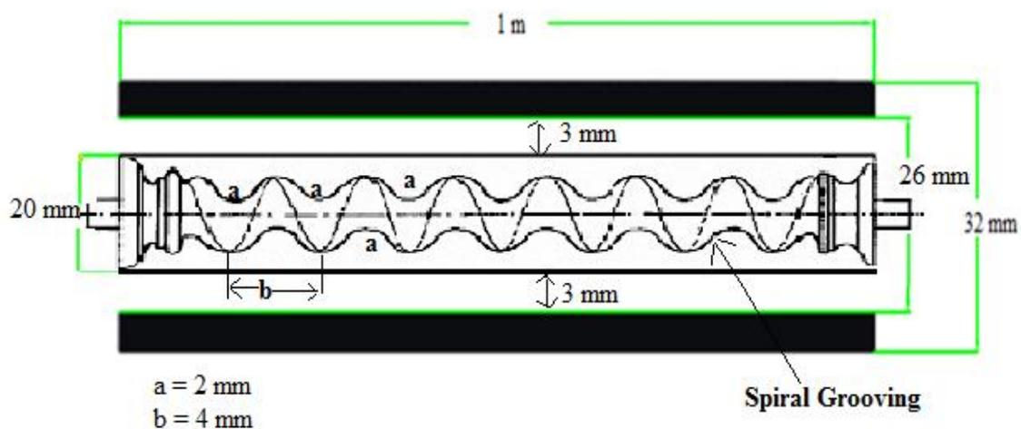
Figure 2: Layout of concentric tube heat exchanger with internal spiral grooving.
