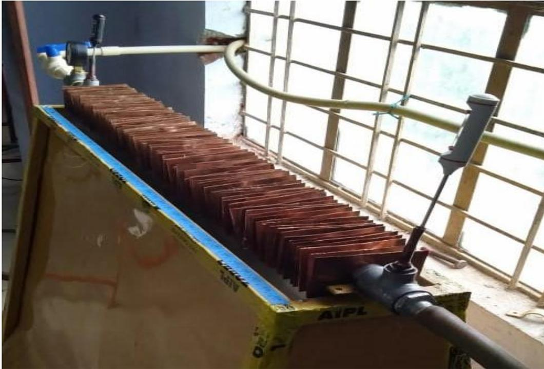
Figure 4: Physical setup for heat exchanger with spiral grooving with rectangular copper fin.
