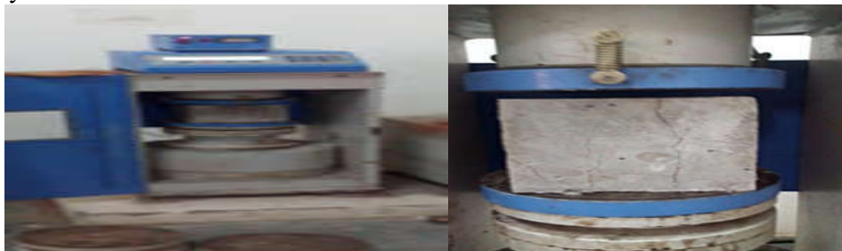
Figure 3.4: Concrete Cubes under Compressive Testing Machine
