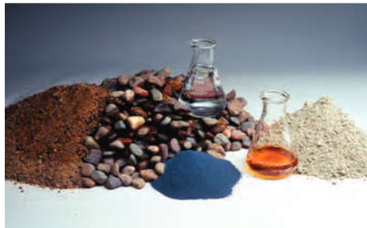
Figure 1.0 Concrete components: cement, water, coarse aggregate, fine aggregate, supplementary cementing materials, and chemical admixtures
