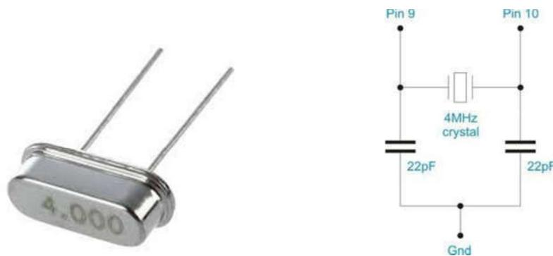
Figure 4: 4MHz Crystal Oscillator and pin diagram
