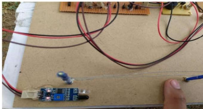
Figure 9: Obstacle detection by IR sensor.
