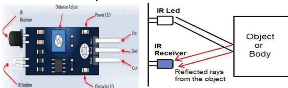
Figure 5: IR sensor components and working
