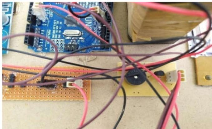
Figure 10: Buzzer alert due to animal detection
