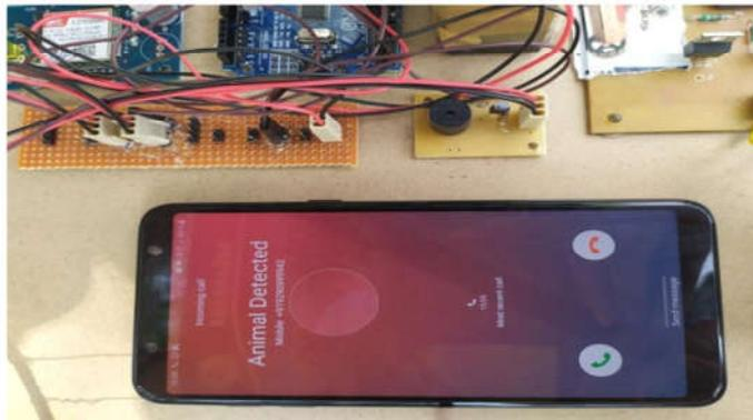
Figure 11: Owner receiving a call via GSM module
