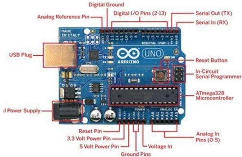
Figure 2: Arduino Uno Microcontroller AT Mega328P
