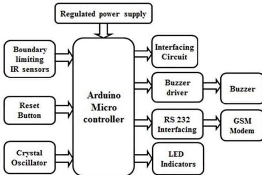
Figure 1: Block diagram of security
