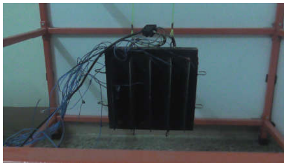
Figure 3. Blackened Plain Aluminium Plate with Rectangular Fins
